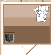
Corner Installation with Protective Cover
