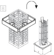
Return the casing with the guard rail into the heater assembly.
