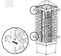
Secure the bracket with screws to the wall.
