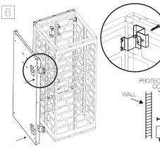
Attach the protective cover 2 together with the wall brackets to the clips in reversse position as protective cover 1.
