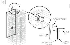
Attach the protective cover 1 together with the wall brackets to the clips.
