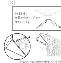
Insert the reflector and bend the legs to the assigned holes on the protective covers to fasten.
