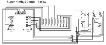
(R11,R21,R22) Temperature Regulator (L1 & L2) Temperature Limiter (H#) Sauna Heating Element (Rly2) Relay # 2, 10A 230 VAC
