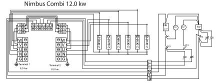
(R2,R3,R4) Temperature Regulato **Temperature Limiter** (L) (Rly1, Rly2) Relay 5A 230VAC (SV) Solenoid valve
