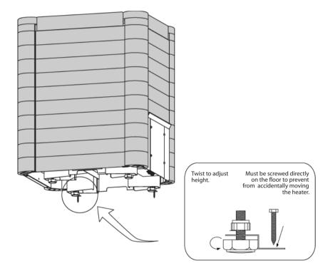
Fig.4 Screwing the Combi Heater on the floor
