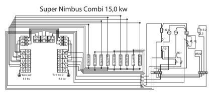
(R1 1,R2 1,R 22) Temperature Regulators(L1 & L2) Temperature Limiter(H#) Sauna Heating Element(Hs1,Hs2) Evaporator Heating Element(Rly2) Relay # 2, 10A 230 VAC(r2) relay 2 contact(Rly1) Relay # 1, 5A 230VA(r1) relay 1 contact
