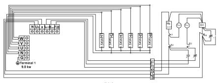
(R2,R3,R4) Temperature Regulator (L) Temperature Limiter (Rly1, Rly2) Relay 5A 230VAC (SV) Solenoid valve
