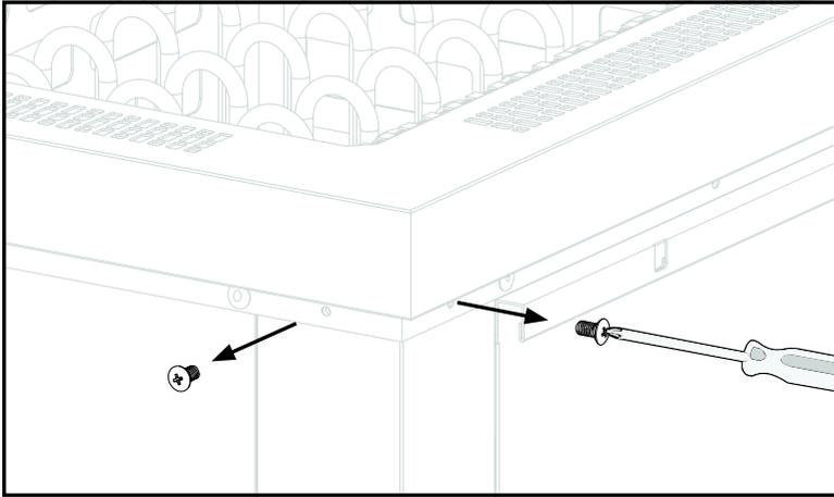
**02** Attach corner and center locks and secure with previously removed screws.
